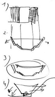
Acting on the safe side, we were committed to the idea of a continuous roof. This solution, however, could not allow enough light for the pitch. The division of the roof in two had then to be faced and tested.
