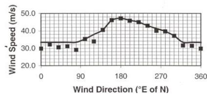
To obtain the "description" of the design wind at the construction site for 100-year return period the data provided by the Merelim Meteorological Station were statistically processed and suitably "corrected" taking into account the "meagre" thirty months of records.
