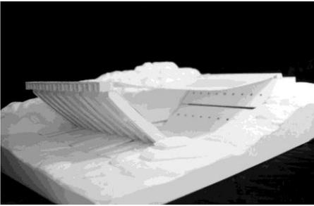
These results showed that the solution with two separate roofs was possible but confirmed the need to develop the analysis of the dynamic interaction between the roof and the wind.
