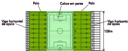
The front edge of the two concrete slabs of the roof support a triangular transversal truss, initially designed as stiffness beam, but modified to accommodate the floodlights and loud speakers.
