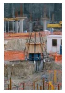
Two pile load tests were carried out. The purpose of the first was to assess the behaviour of the piles under maximum load. (2 x the service load on a Ø800 pile). The second test was aimed at evaluating the pile's inservice behaviour (1.5 x service load on a Ø1300 pile). The results of the load tests confirmed that the piles had been properly built. Note that the load tests were carried out when the job was already underway (they were not prior tests).
